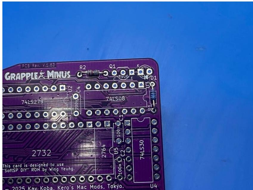
2. Next, solder the Q1 3906 Transistor to the PCB. Make sure the flat side is facing up.
