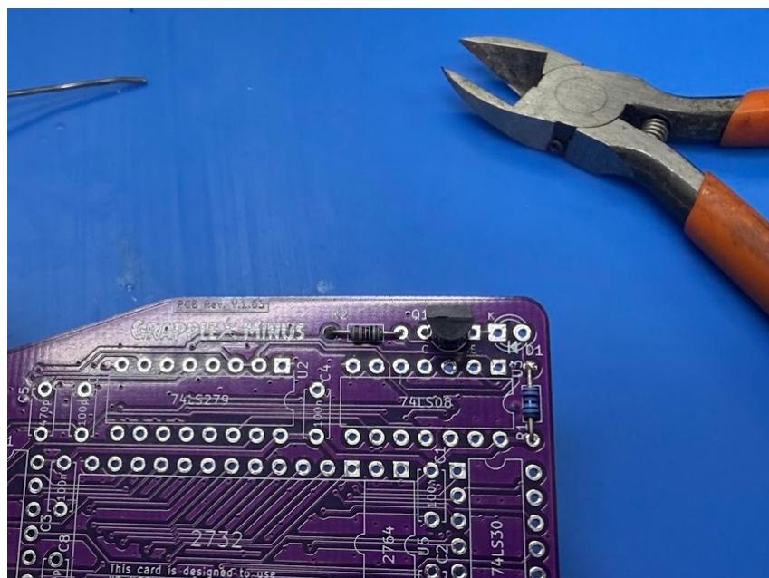
3. Next, solder the LED. The side marked with a "K" on the PCB silkscreen will be the cathode, so align the shorter leg of the LED with the K.
